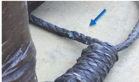
Detail of green corrosion on noose.
